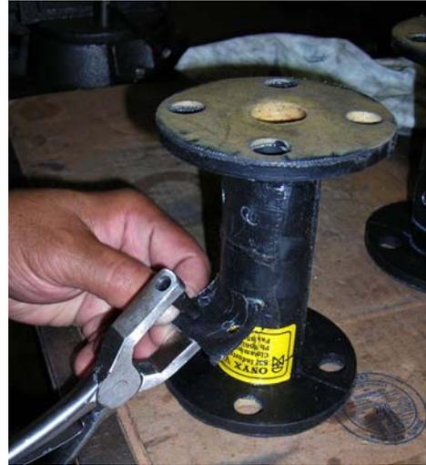
b) Punch holes through the Positive Opening Tabs using a gasket hole or pliers type punch. Hole diameter in tabs should be approximately equal to hole diameter in the pinch bar.
