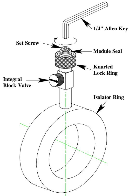
Turning the Module Seal Set Screw clockwise eliminates weeping but makes the fit around the needle tighter.
