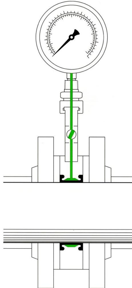
If you detect instrument oil weeping from under the Lock Ring, the Module Seal may require minor adjustment.
