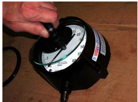
Figure 3: Remove the lens from the gauge.
