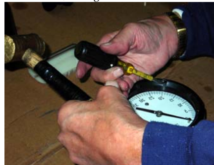
Figure 2: Tapping the bezel ring.
