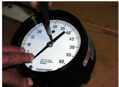
Figure 4: Re-zero the pointer.
