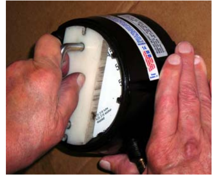
Figure 1: Use a bezel wrench to remove the bezel ring
