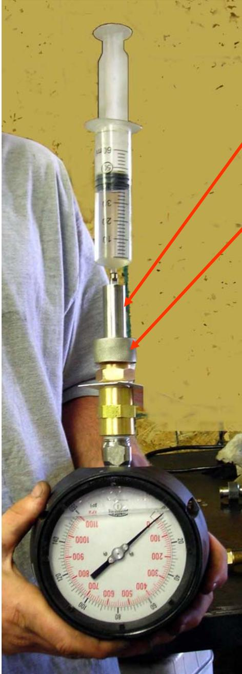
1. Attach a Stinger Fitting to the gauge or other pressure sensing instrument.
