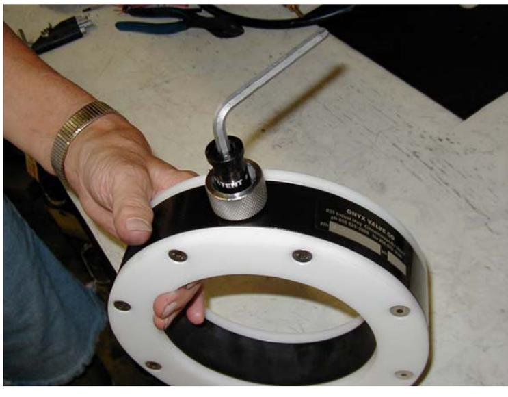
If the module seal is too tight to insert the stinger fitting, loosen the adjustment a little bit by rotating the hex key anti-clockwise. Just a few degrees of rotation with the hex key should be sufficient to reinsert the stinger.
