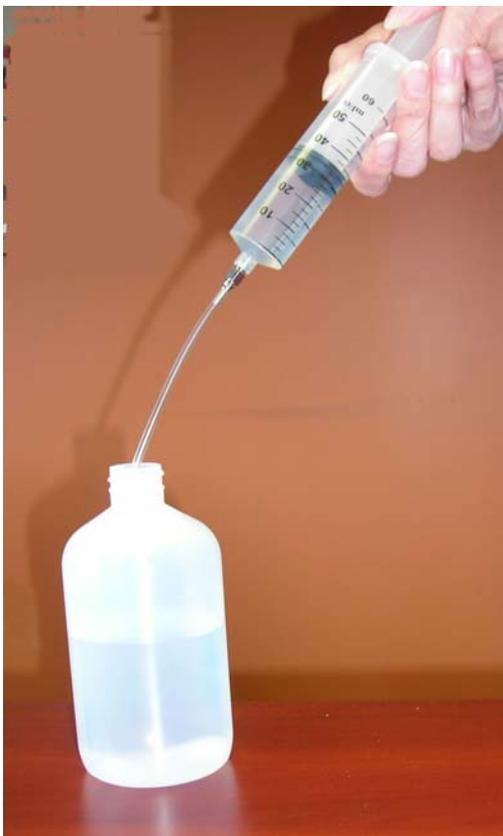
Attach the Proboscis fitting to the syringe.
