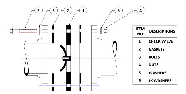
2. For horizontal pipeline, install valve with the clamp plate in vertical upright position.
