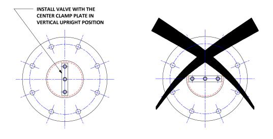
3. For vertical pipeline, valve can be installed **Flow Up** direction only.
