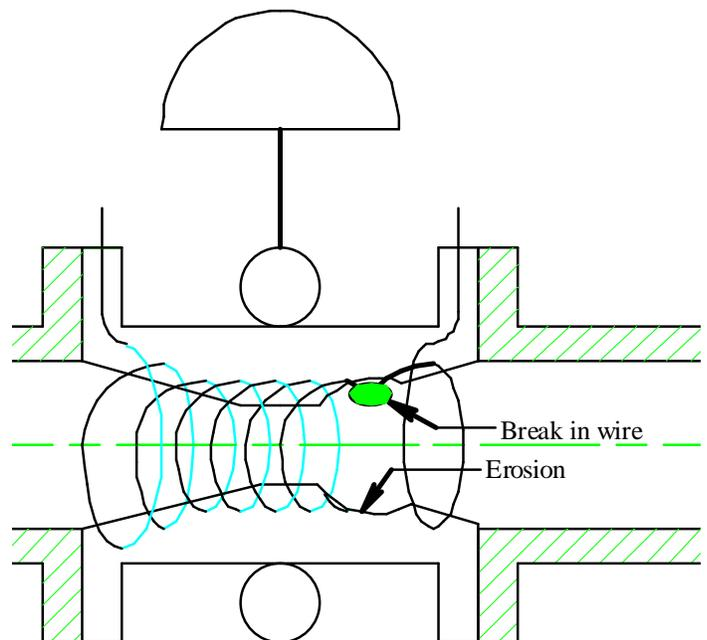
But this situation can get stickier: What if the piping in the plant is grounded (as it normally is)? In this case, when the wear-wire is exposed to the process fluid, the I/O electric potential is shorted directly to ground.
