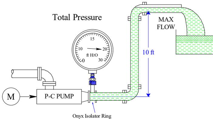
**Total pressure = Static Pressure + Friction Pressure.**
