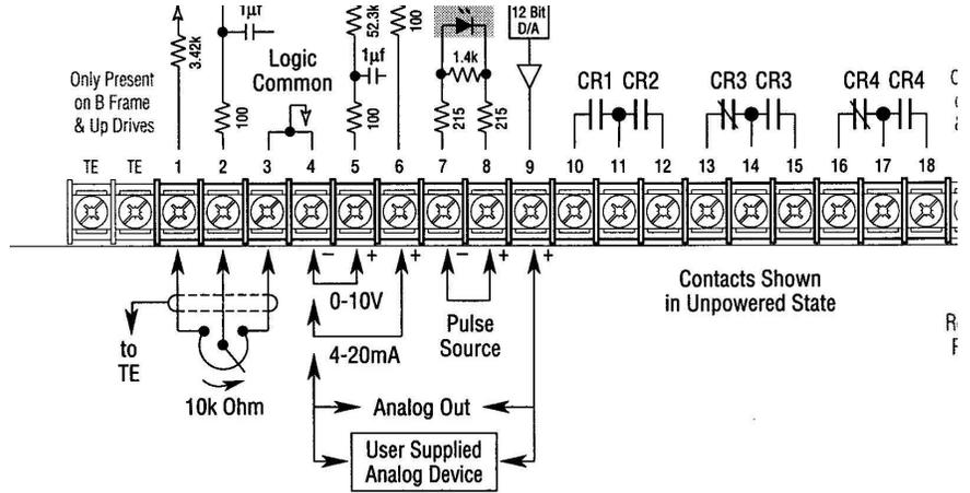
In our example we used CR-1 as the run relay. Connect terminal #10 in the A-B drive to Smart Box terminal #2. Connect terminal #11 in the A-B drive to terminal I-1 in the Smart Box.
