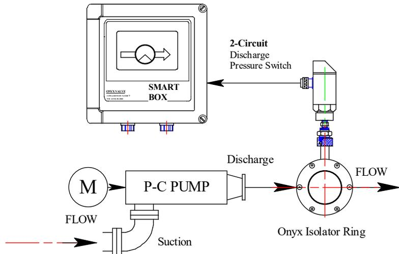
How can you protect a pump against **BOTH** Over-Pressure and Run Dry with **1** Switch?
