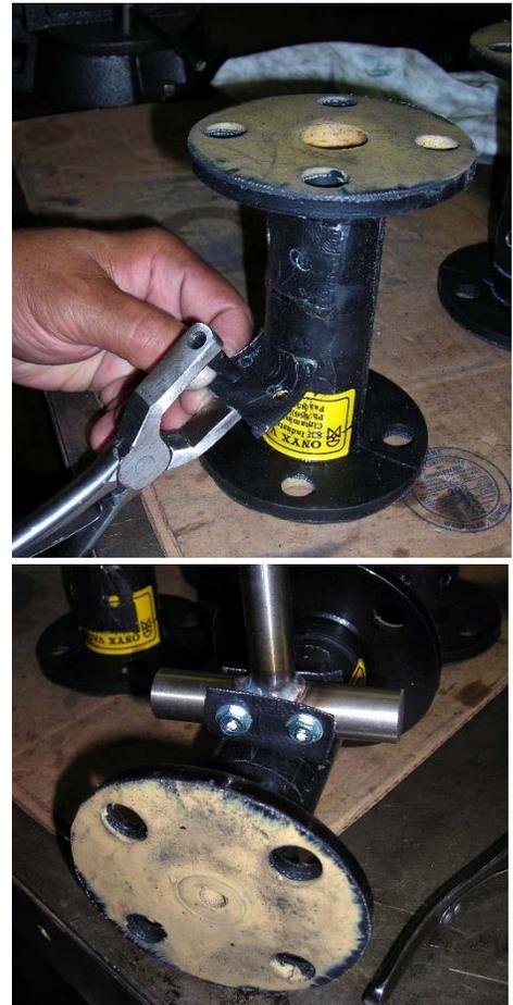
10. If valve is provided with optional bonnet seal kit, loosen the spud nut (#12A) and yoke adapter (#12) and replace O-rings (#12B & 12C).
