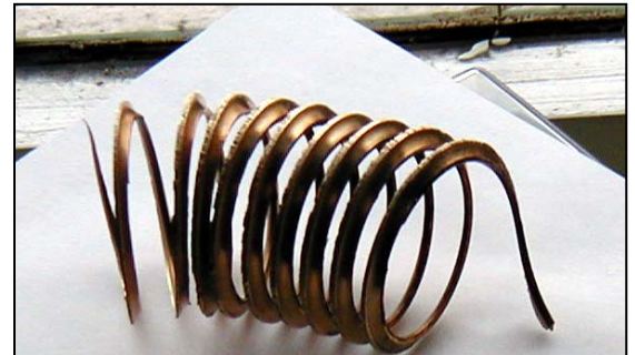
The dreaded “Slinky “effect: This used to be the threads in an electric actuator drive nut.
