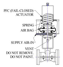
It has a sintered metal breather vent on the bottom. Actuator cannot operate properly if this vent is not functional.
